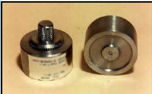
The Graduated Grinding Jig is used for grinding discs to accurate, predetermined, thicknesses prior to electropolishing.
