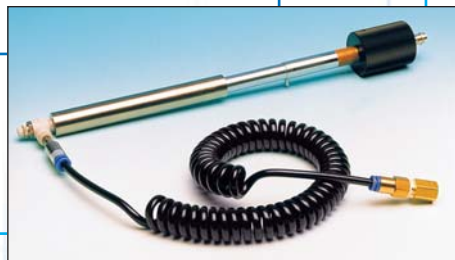
Vacuum Storage Container for specimen stage storage and transfer.
