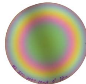
4" Glass disk deposited with ITO coating using the IBS/e-KDCDEPO
