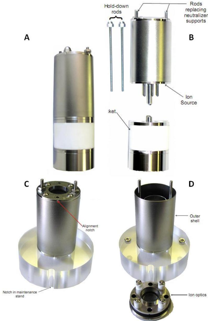
**Figure 5 Ion Optics change for the KDC-10 Ion source.**
