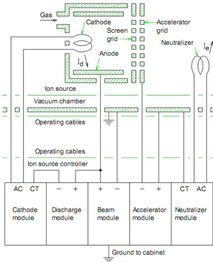
Figure 1 Electrical schematic of a Kaufman ion source.
