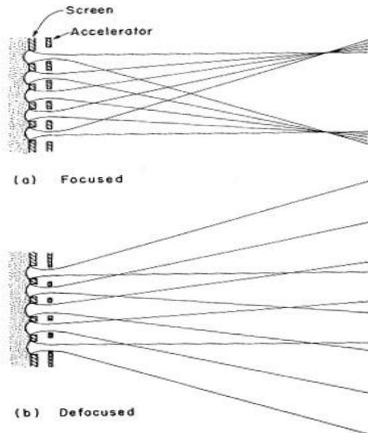
Figure 3 Ion grid optics for (a) Focused and (b) Defocused conditions.
