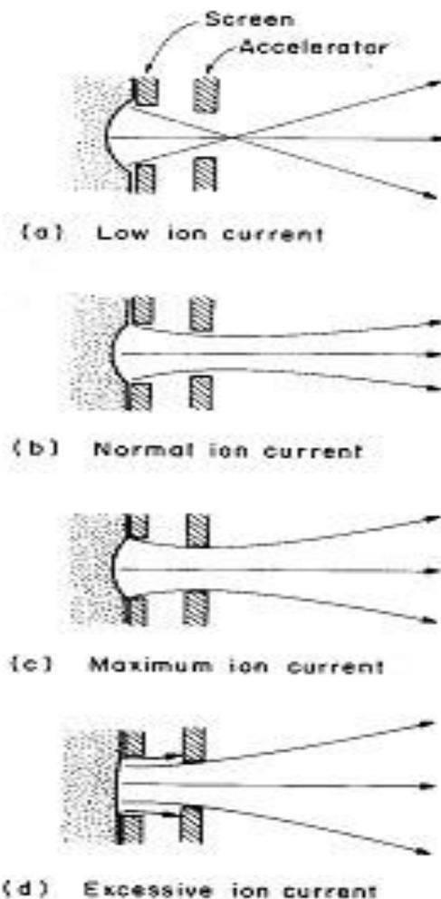
**Figure 2 Multi-aperture grids with different current conditions.**
