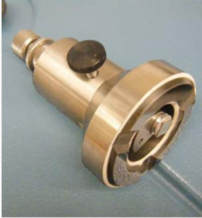
Two SEM pin mount stubs can be mounted into a modified specimen mount to fit an SBT model 150 micrometer controlled lapping fixture for polishing. The specimen remains attached to the stub during polishing and can be transferred directly to the SEM or stored and transported in the SampleSaver™ storage container.
