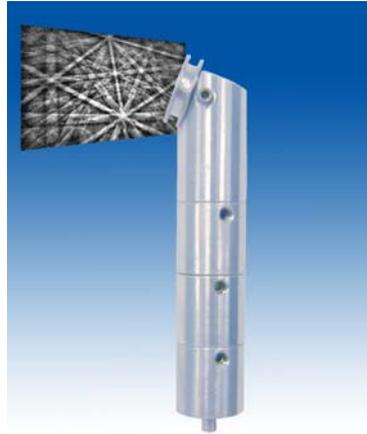
Pre-Tilt EBSD specimen stage with multiple height adjustment segments. Samples are kept at fixed 70° or 20° for EBSD analysis. The stage can be stored with a specimen in the SampleSaver™ storage container.
