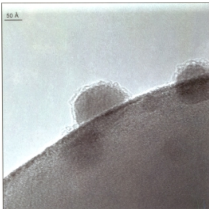
Figure 5: TEM image of Pd/SiO 2 particles deposited with 8Å of tungsten film using the Model IBS/e. From the image it is clear that the film is thin, continuous, amorphous, and uniform over the entire sample area. (Image courtesy of L. Allard, Oak Ridge National Lab and D. Joy, University of Tennessee)
