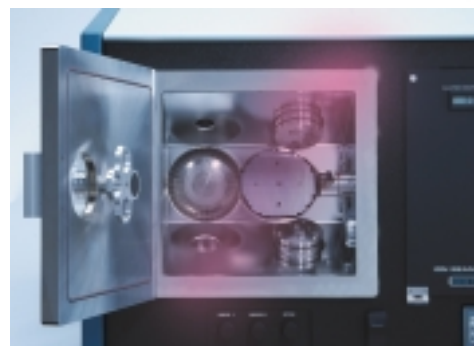
Figure 1: The Model IBS/e Ion Beam Sputter Deposition and Etching System. The inside of the vacuum chamber is shown at right with the Large Area Stage (LAS) installed. Targets are mounted to the chamber lid and can hold up to 4 different target materials.
