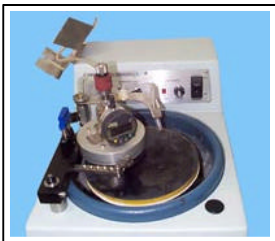
Figure 1: Illustration of the lapping and polishing setup used for processing. The Model 920 Lapping and Polishing Machine is shown with the Model 92002 Workstation and the Model 147D Lapping and Polishing Fixture. The system uses an 8" diameter lapping wheel combined with abrasive suspension or polishing cloth to produce a lapped, smooth surface.
