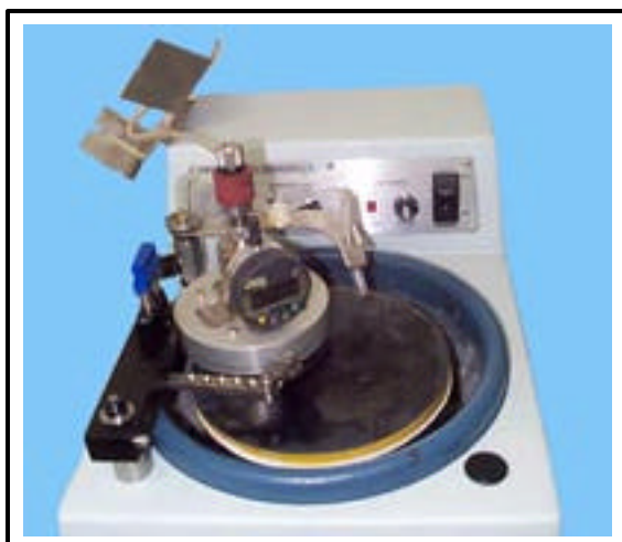
Figure 3: Illustration of the lapping and polishing setup used for processing YVO 4 . The Model 920 Lapping and Polishing Machine is shown with the Model 92002 Workstation and the Model 147D Lapping and Polishing Fixture. The system uses an 8” diameter lapping wheel combined with abrasive suspension or polishing cloth to produce a lapped, smooth surface.
