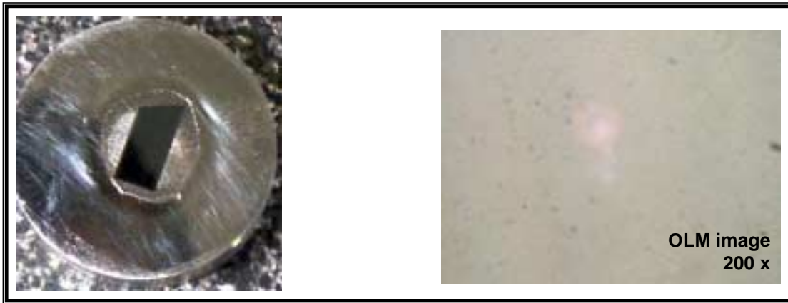
Figure 1: Illustration of the final polished surface of the silicon samples following processing. On the left is the specimen as mounted on the fixture stub and the right shows an OLM image of the surface after processing.
