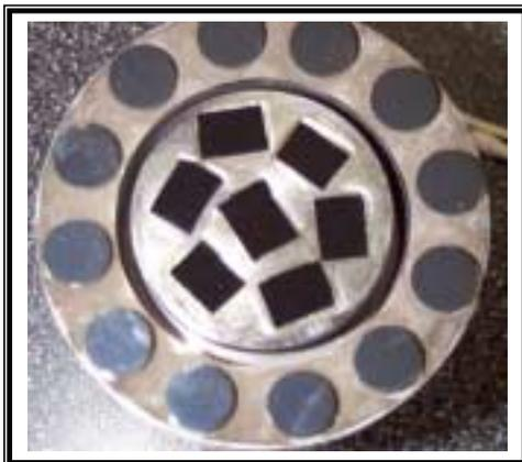
**Figure 10:** Image showing the final polished surface of the silicon die following processing. Note the specular surface and the high polish quality obtained using this process.
