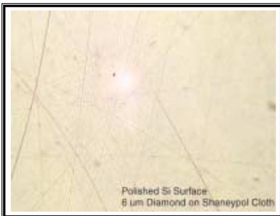
**Figure 7:** Image of the polished surface of silicon following polishing with the ShaneyPol polishing cloth and 6  $\mu\text{m}$  diamond slurry. The surface of the specimen is free of mechanical damage from the lapping process and shows only surface scratches from the 6  $\mu\text{m}$  abrasive media.
