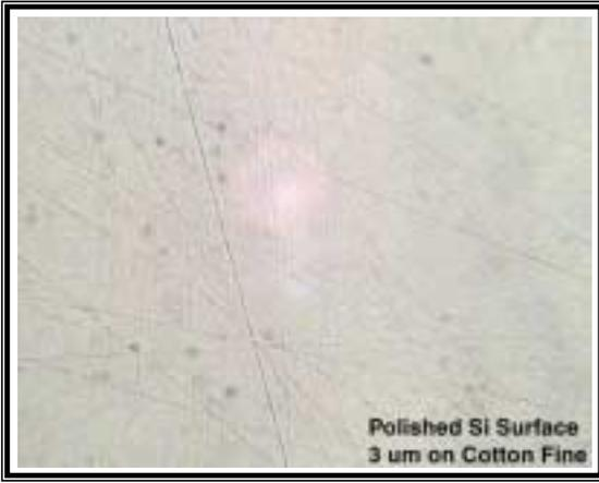
**Figure 8:** Image showing the Si surface following polishing using the Cotton Fine polishing cloth and 3  $\mu\text{m}$  diamond slurry. Note the scratches on the surface which correspond to the 3  $\mu\text{m}$  abrasive size with no visible pitting or mechanical damage present from the lapping process.
