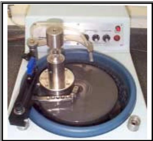
**Figure 1:** Setup used for lapping and polishing specimens in this experiment. A Model 920 Lapping and Polishing Machine is shown equipped with a Model 92002 Workstation and Model 155 Lapping and Polishing Fixture. The Model 155 is shown captured in the Model 92002 and is continuously rotated counter-clockwise. The lapping wheel also rotates counter-clockwise and is variable speed up to 600 rpm.
