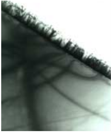
Figure 3: XTEM image of a GaN film on Sapphire prepared using the Tripod Polisher® followed by ion thinning at low angle. As can be seen the image shows electron transparency through a wide range and exhibits thin areas both in the GaN film and Sapphire substrate.
